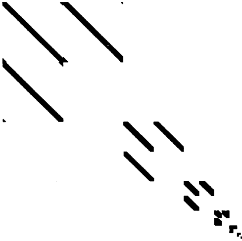
FIG. 5. NS-form representation of the operator A^{-1}B used in the Crank–Nicolson scheme (5.12). Entries of absolute value greater than 10^{-8} are shown in black. The wavelet basis is Daubechies with M = 6 vanishing moments ( L_f = 18 ), the number of scales is n = 9 and J = 7 . We have set \nu = 1.0 and \Delta t = \Delta x = 2^{-9} . Note that the top left portion of the figure contains nonzero entries which indicate high frequency components present in the operator A^{-1}B .
